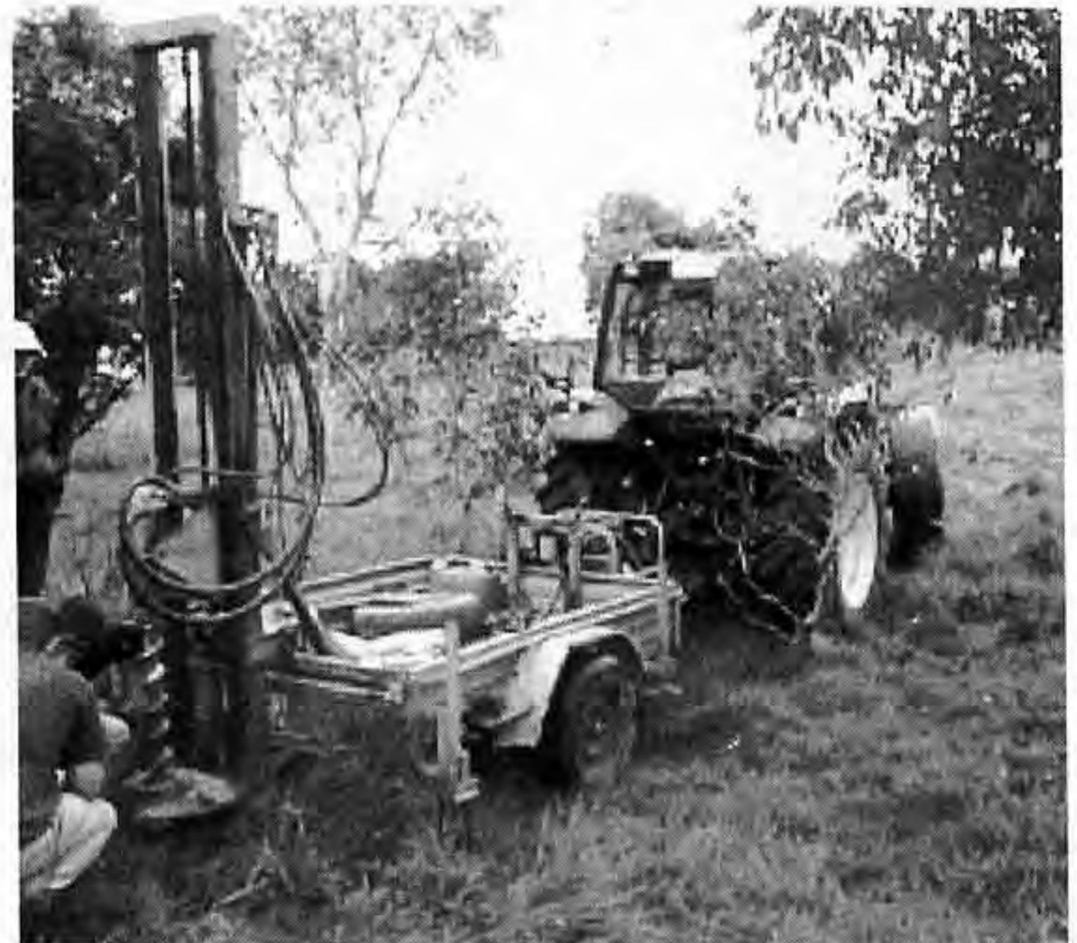
Taking a borehole soil sample with a power auger.
